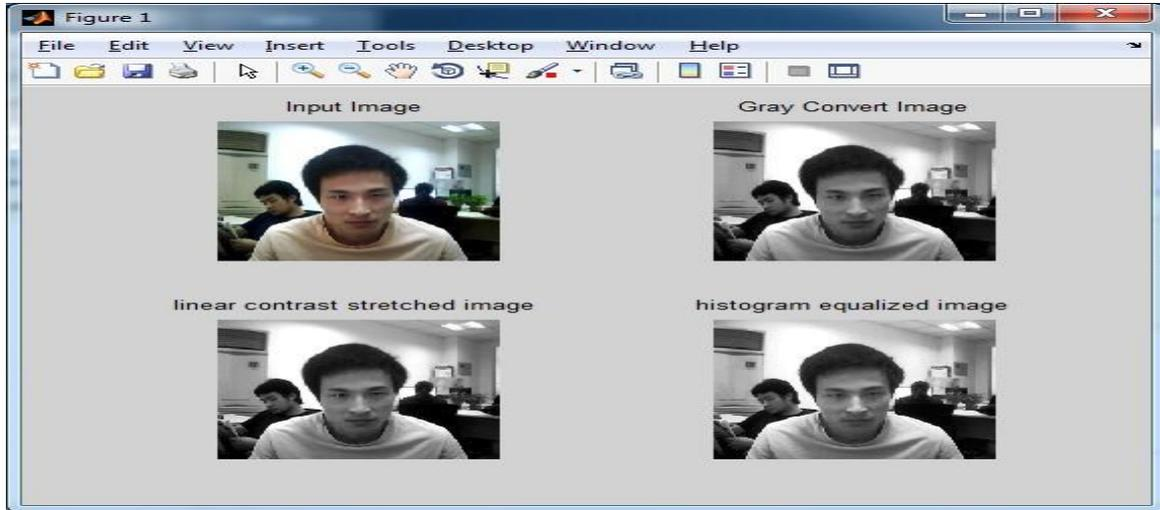
**Fig. 2 Input (Real) Image, Gray Convert Image, Linear Contrast Stretched Image, Histogram Equalized Image**
