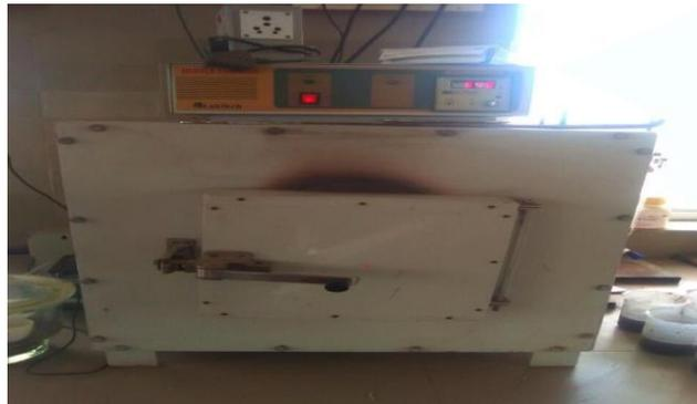
Fig 6 Muffle furnace
