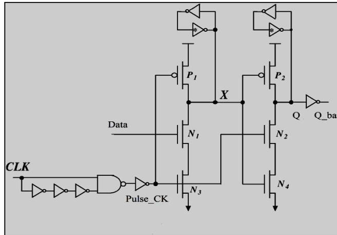
**Fig.1. Explicit pulse triggered Data close to Output**
