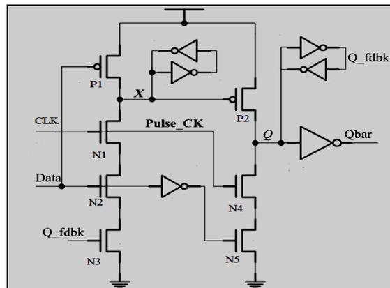
**Fig.3. Static Conditional Discharged Flip - flop**
