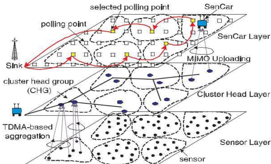
**Fig 1. Illustration of the LBC-DDU framework**
