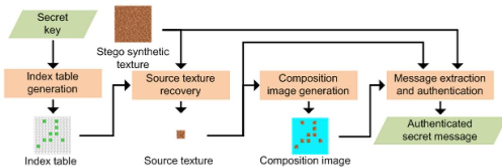
Fig. (b) Message Extracting Procedure
