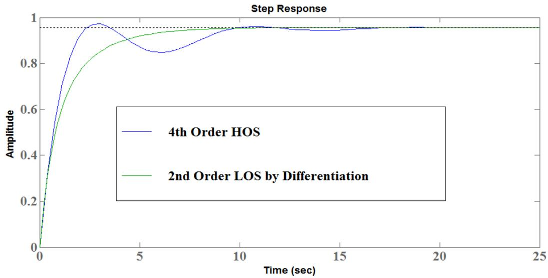
Fig.7. comparison of step responses of HOS (4<sup>th</sup> order) and LOS (2<sup>nd</sup> order).
