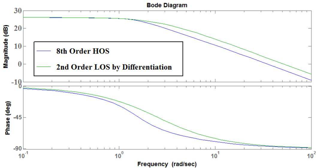
Fig.2. Comparison of Frequency Responses of HOS (8<sup>th</sup> order) and LOS (2<sup>nd</sup> order)
