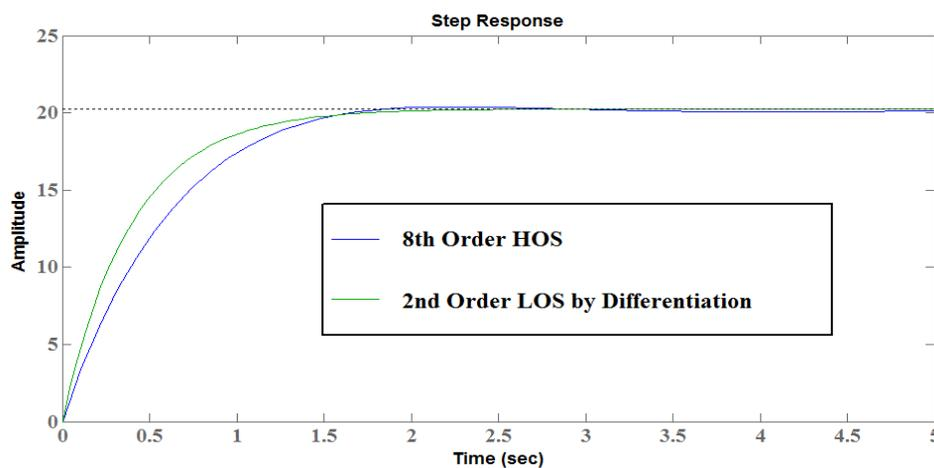
Fig.1. Comparison of Step Responses of HOS (8<sup>th</sup> order) and LOS (2<sup>nd</sup> order)
