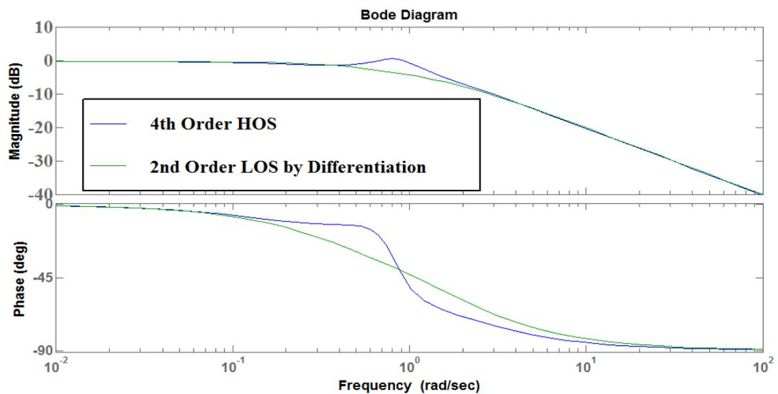
Fig.8. comparison of frequency responses of HOS (4<sup>th</sup> order) and LOS (2<sup>nd</sup> order).
