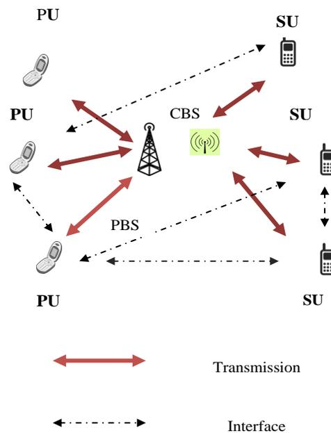
Fig.1 System model of OFDM based cognitive radio system
