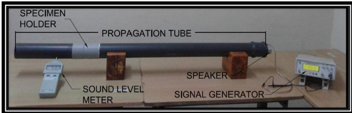
Fig.2 Experimental Set up for Noise Absorption Measurement
