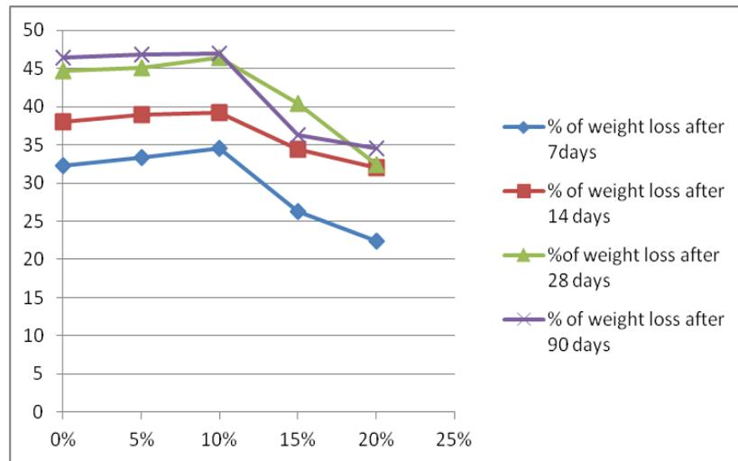
**Graphical representation for percentage loss of weight after treating with 2% of mgso<sub>4</sub> in hypo sludge after 7, 14, 28 & 90 days curing**
