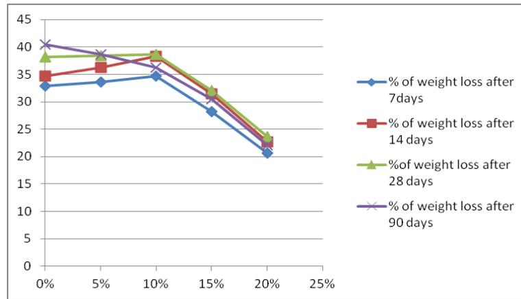
Graphical representation for percentage loss of weight after treating with 3% of Mgso4 in ceramic waste after 7, 14, 28 & 90 days curing
