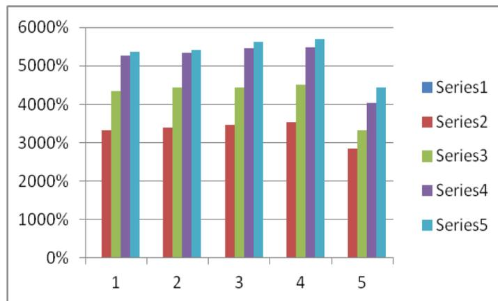
**Graphical representation of comparison between 7, 14, 28 & 90 days compressive strength values for replacement of cement by hypo sludge**
