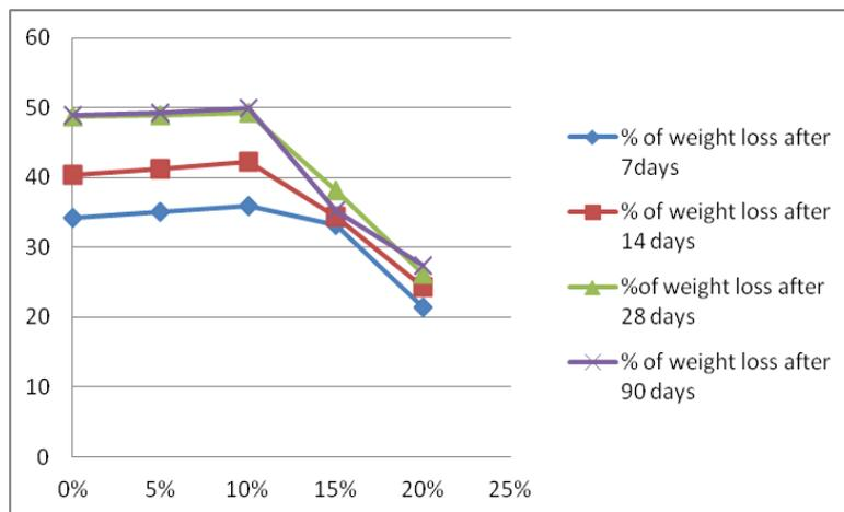
Graphical representation for percentage loss of weight after treating with 1% of Mgso<sub>4</sub> in ceramic waste after 7, 14, 28 & 90 days curing
