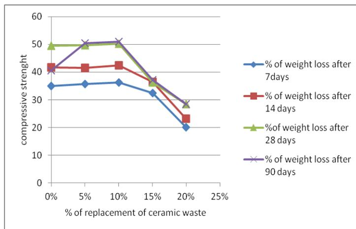
**Graphical representation for percentage loss of weight after treating with 2% of mgso<sub>4</sub> in ceramic waste after 7, 14, 28 & 90 days**
