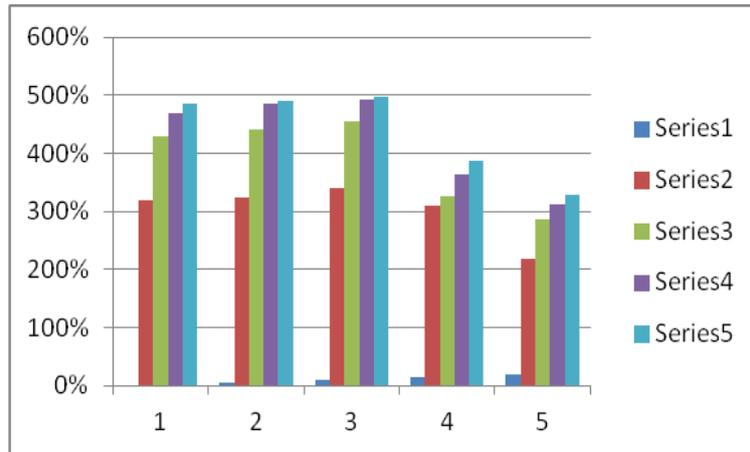
Graphical representation of comparison between 7, 14, 28 & 90 days split tensile strength values for replacement of cement by hypo sludge
