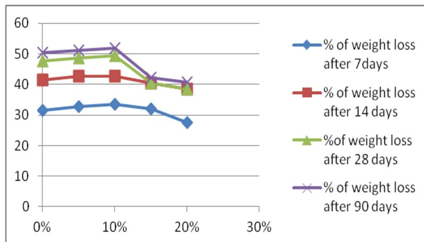
Graphical representation for percentage loss of weight after treating with 1% of mgso4 in hypo sludge after 7, 14, 28 & 90 days curing
