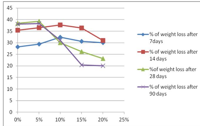
Graphical representation for percentage loss of weight after treating with 3% of mgso<sub>4</sub> in hypo sludge after 7, 14, 28 & 90 days curing
