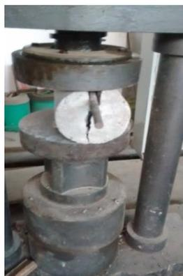
*Fig.4 Specimen subjected to Split tensile strength*
