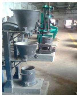
*Fig.3 Compaction factor test*
