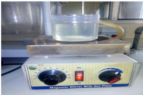
Fig.6 Nano lubricant on magnetic stirrer
