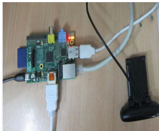
Fig 4 . Connection of USB Camera With Raspberry Pi
