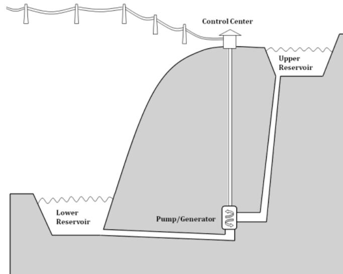
**Fig.1: Pumped hydroelectric storage system**
