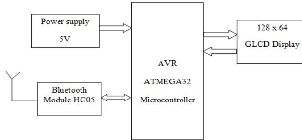
**Figure 2: Transmitter unit**
