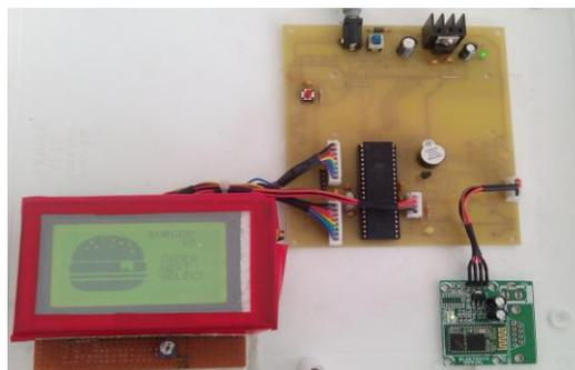
**Figure 8: Image of touch screen based ordering system**
